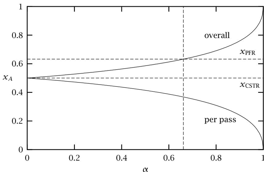
**Figure 4.27:** Overall and per-pass conversion of A as a function of fractional recycle,  $\alpha$ .
