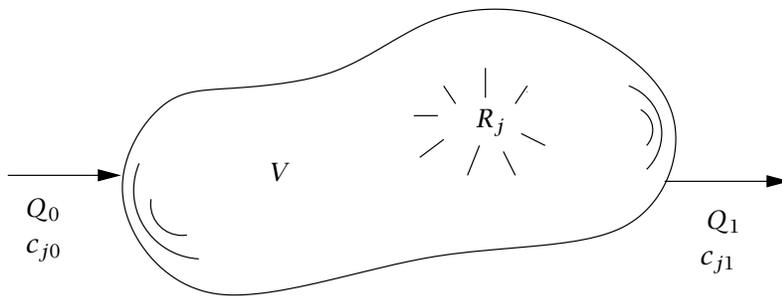
Figure 4.1: Reactor volume element.
