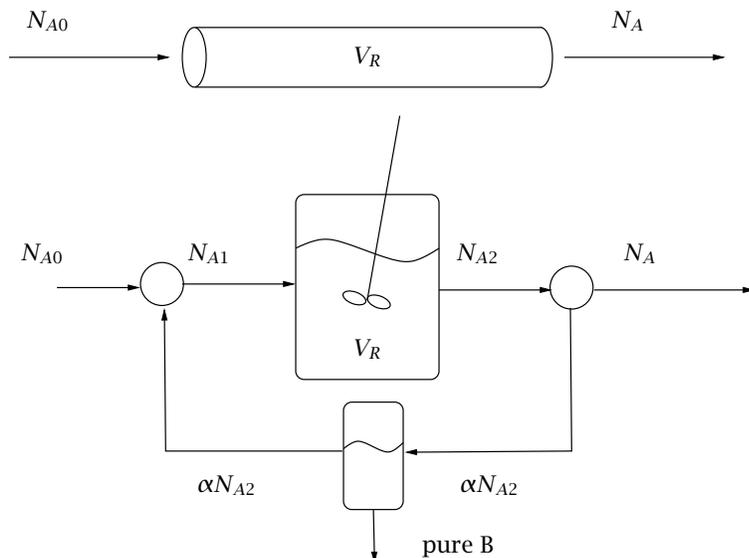
**Figure 4.26:** PFR versus CSTR with recycle and separation.
